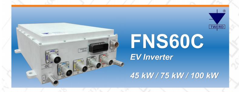
**FNS60C** electric vehicle inverter (EV Inverter) is a motor controller for electric vehicles. This electrical device converts electricity between a DC (Direct Current) circuit on battery side and AC (Alternating Current) on electric motor side. EV inverter controls the operation of the electric motor (an example: start/stop, forward/reverse rotation, selecting and controlling the speed, modifying or limiting the torque) and protecting against faults and overloads.
