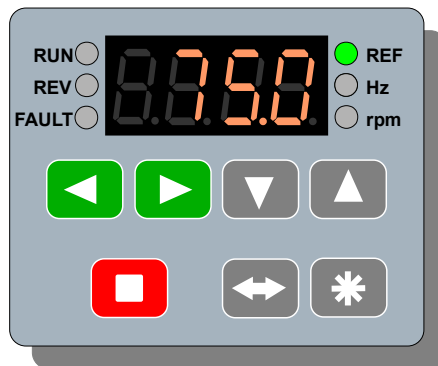
Fig. 6.2. Changing the PI controller ref.-unit value (keyboard ref.-unit: par 2.60 = 0)
